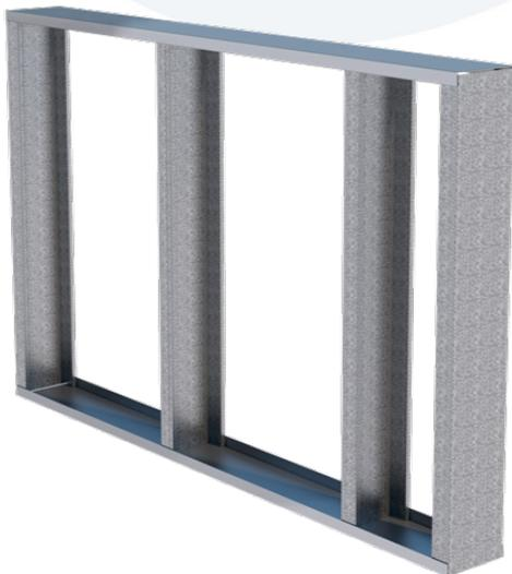
Taller parapets are usually formed by infilling Ayrshire sections between hot rolled posts. These posts are often spaced at 3m or 4m centres. Longer spacings can be achieved but may require an Ayrshire boxed section at the head of the parapet.
