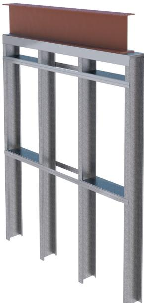
The traditional deflection head system uses Ayrshire's UR head track fixed to the structural frame above. The studs slide into the head track but are not fixed directly to it. A line of bracing & blocking is installed to the studs, 150mm down from the top of the panel, to prevent racking of the studs.
