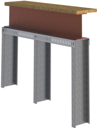
The slotted head track is an efficient system that minimises the number of components & increases the speed of erection. Ayrshire's URS head track is fixed to the structure above and features slotted holes in both flanges. Fixings are positioned at the mid-height of the slot & screw into the stud behind.
